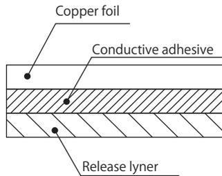
Thin and flexible metal foil tape backed by a conductive filler adhesive
