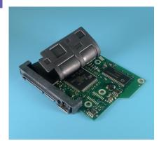
Injection-moldable, thermally conductive elastomer
